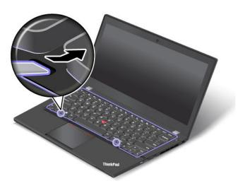
4. Tighten the screws with the keyboard multi-tool to secure the keyboard in place.
